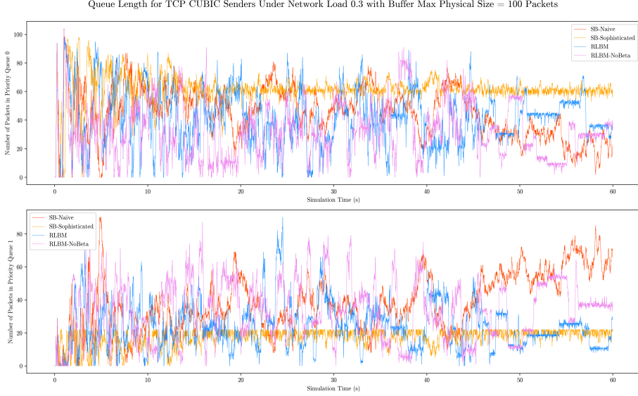
Figure 13: Queue length over the course of the simulation, configured as specified. We observe that the queue length never exceeds the physical maximum size (100 packets). Moreover, observe the impact of the fixed per-queue \alpha weights in the Static Buffer Schemes, with the length of the Priority 1 queue being practically limited by the buffer capacity and the 8\times \alpha weight of the Priority 0 queue.
