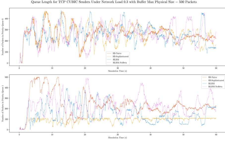
Figure 14: We begin to more clearly observe the difference between the RLBM scheme with pre-determined \beta weights and without; the RLBM: No \beta scheme allocates more buffer space to the Priority 1 queue than the RLBM scheme.
